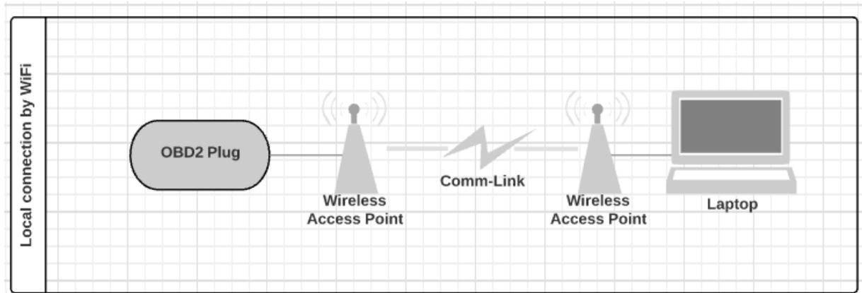
In this scenario car is connected to wireless access point which is connected in client mode to another AP and then to PC. Depending AP configuration (DHCP server enabled or not) the IP-assignment can be done by AutoIP or DHCP. Both car and PC has to be in same network segment to enable the UDP broadcasts
