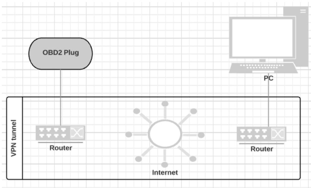
Advanced topology. The local network is connected to remote network using VPN-Tunnel, which logically extends local network to remote location. You can then diagnose a car located hundreds kilometers away exactly in the same way like in local garage. Many modern routers have VPN functionality built-in, in other case
