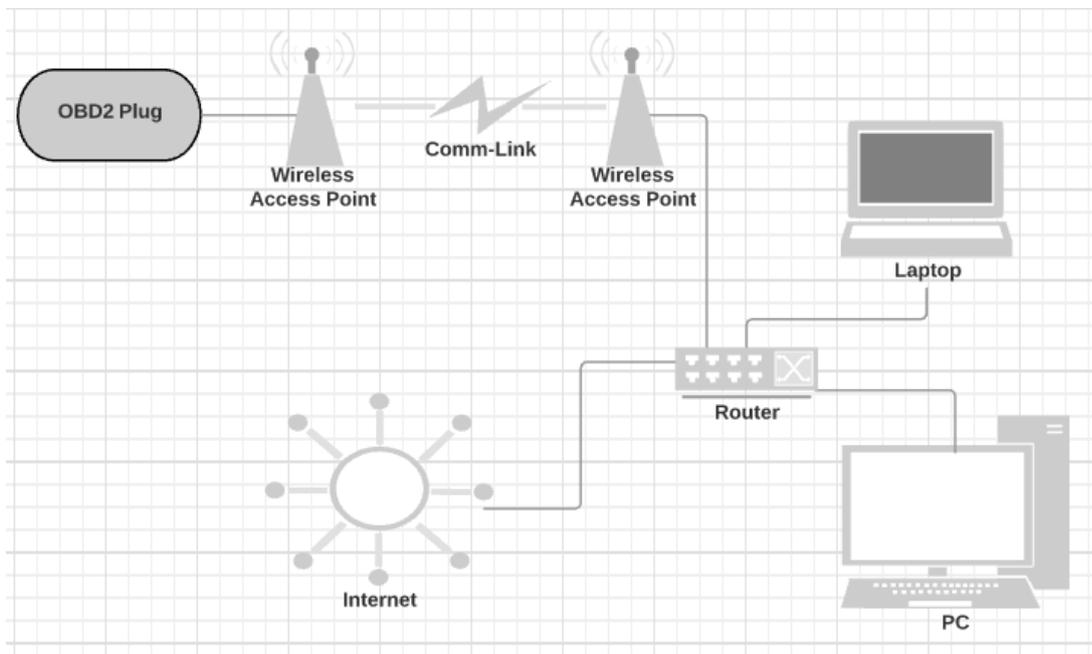
Typical network diagram in small offices, workshops etc. This time router is responsible with DHCP-address assignment, the AP in client mode then connects car to rest of the infrastructure. Then VCP installed in PC or laptop will be able to communicate with a car.
