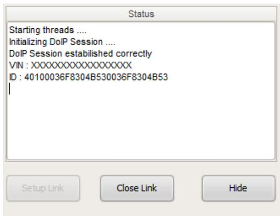
Once connection is established, you can hide the window using "hide" button and use VCP in the regular way. All functions (diagnose / flash / parametrization / scripiter) work with DoIP.
