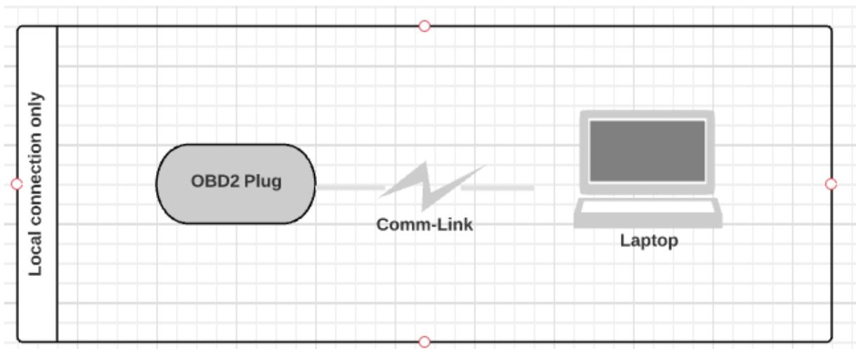
In this scenario car is directly connected to your PC. IP-Assignment is done by a AutoIP standard which is fully supported by Windows OSes. Make sure that any software-Firewall will accept incoming and outgoing connections to port 13400 UDP and TCP
